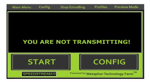
This is the Start Point to Broadcast Kit Operation. If you do not see this screen when the Kit starts, you must remove the modems then restart the Kit.
